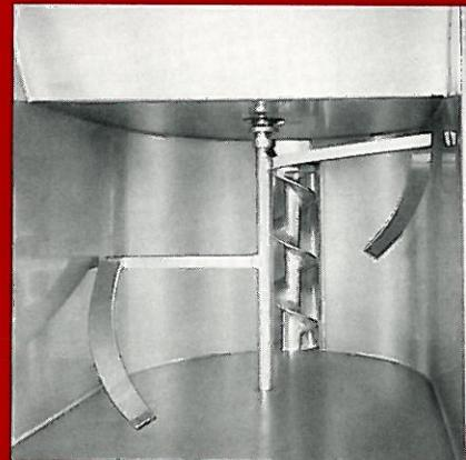
Top View of Mixing arm and feed screw. Mixing arm moves product forward to assist the feed screw in fast, consistent emptying of the entire load of product.
